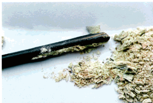
Figure 8. Degradation of the black PrAlO 3 –Pr 2 O 3 eutectic rod into a yellow fine powder, after ca. 1 week of exposure to air.
